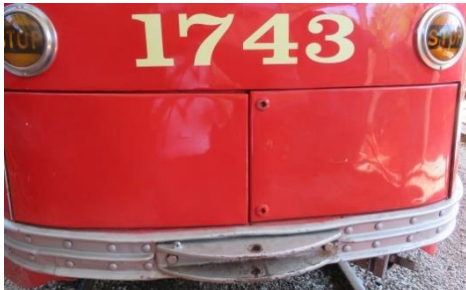
Battery Compartment On Rear of Streetcar
